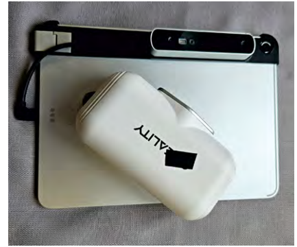
16 Ipad with add-on scanner, hand scanner.
