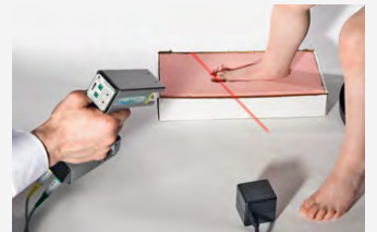
Fig. 13 Scanning the foot in the foot foam.
