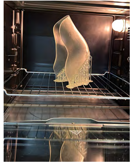
4, 5 The final strength of the printed object is only achieved by post-exposure in the curing box (left) and by thermal post-treatment during tempering (right).
