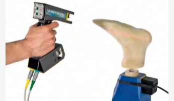
Fig. 12 Scanning a positive shoe last (manufacturer: Spenle).
